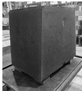
Fig.4. Industrial scale block of approximately half a ton prepared with BestDrying TR bonded castable after fast drying test.
