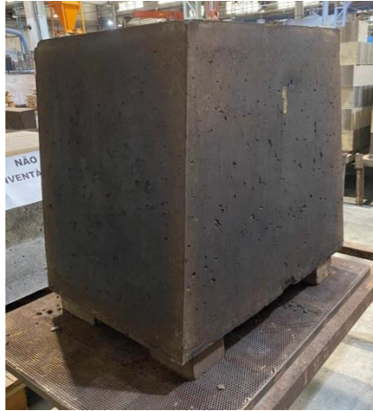
Figure 5. Industrial scale block of approximately half a ton prepared with Fastfrax® bonded castable after fast drying test.
